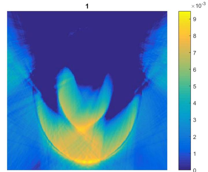
*Tomographic reconstruction of wrapped phase data via the phase-SIRT algorithm*
